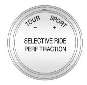
This knob is located on the center console. Turn it to select the suspension of your choice. The knob will return to the center position when released. The switch will illuminate the current suspension setting.
